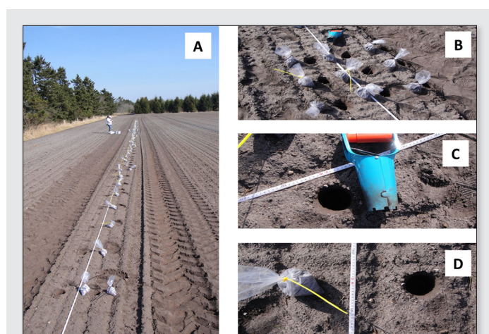
Figure 2. Sandy soil sampling. a) Long range profile for variographic characterisation (~100m) parallel to the recent ploughing direction; b) Local "grid replication design" (9 samples covering 1 × 1 m); c) Conventional soil sampling hand tool; d) Sample excavation and airtight sample bag.
