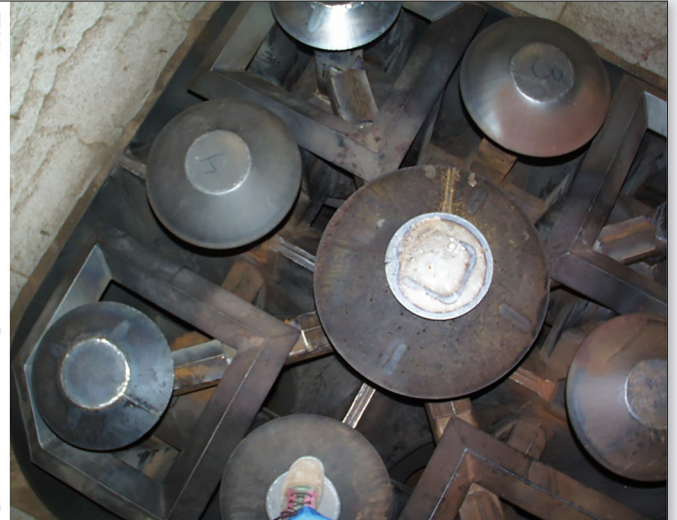
Figure 1. Schematic drawing and photo of a Nierns shaft cooler. Material falls from the kiln head into the top of the cooler. Cooling air is blown in from below as shown in the drawing (left).
