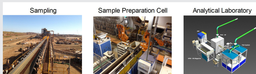
Figure 1. The three components of the Cape Lambert Port B automated sampling and analysis facility [1].
