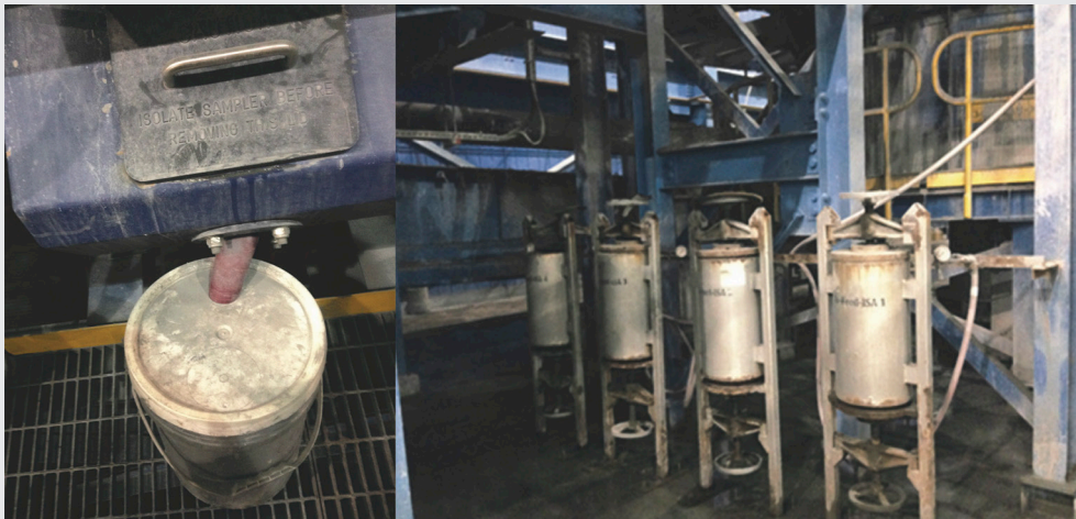
Figure 5. Typical bucket sampling system with manual filter presses.
