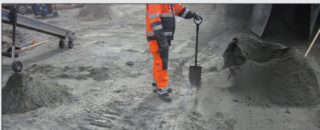
Figure 14. Visual comparison of primary sampling belt collected drill cuttings pile on the left vs. the remainder of the blast hole cone after 14m drilling.
