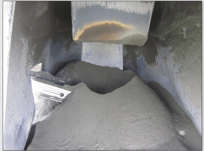
Figure 12. A drill cuttings cone as viewed from under the dust curtain, with the RAS conveyor belt in place.
