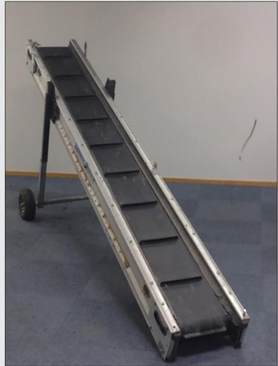
Figure 3. Primary sampling belt conveyor used in this study. Conveyor width was 400mm and length 3 meters.
