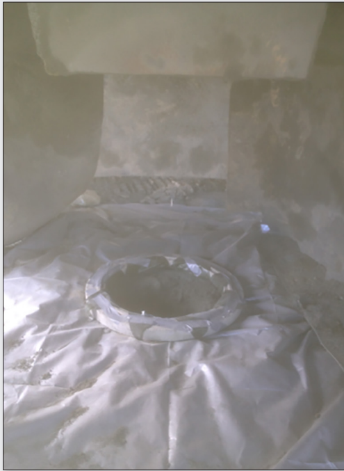
Figure 10. Tarp laid on the ground around the concrete ring, which surrounds the blast hole.
