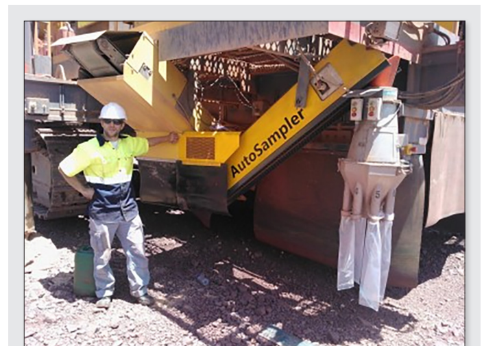
Figure 1. RAS – Rotary Autosampler installed in a rotary drill
