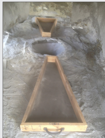
Figure 15. Triangular sampling trays next to the blast hole prior to drilling 3 meters.
