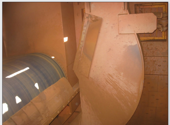
Figure 11. Cross-stream cutter with a large cutter body to eliminate sample reflux at high flow rates.
