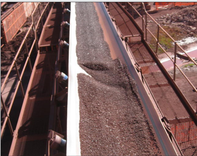
Figure 14. Sample cut taken by a cross-belt sampler indicating that a full cross-section of ore was not removed from the conveyor belt.
