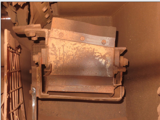
Figure 12. Poorly designed and maintained secondary cross-stream bucket cutter resulting in sample loss during its traverse.
