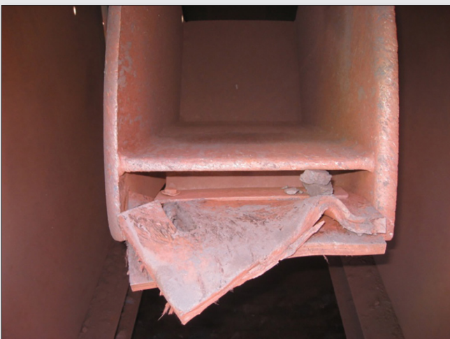
Figure 15. Poor condition of the rubber skirt on the bottom of a cross-belt cutter.
