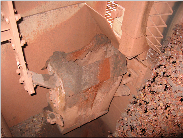
Figure 16. Excessive sample build-up and partial blockage of a secondary cutter aperture.
