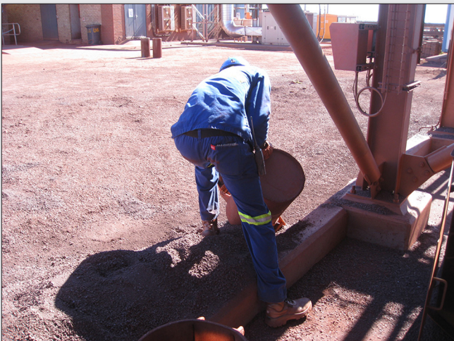
Figure 2. Accessory error caused by an operator tipping out part of a sample on the ground instead of using a rotary sample divider or a riffle to reduce its mass. The supervisor is not doing his/her job.
