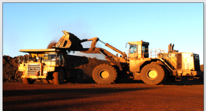
Figure 4. Reclaiming of pre-crusher stockpile for transport to the crusher.
